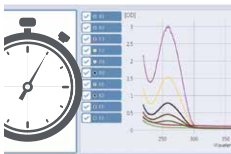
Fast absorbance scan of a Didymium filter from 200-1000 nm with 1 nm resolution
