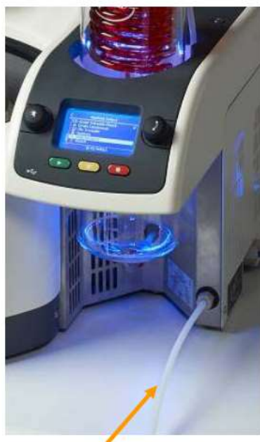
Waste solvent drain hose
