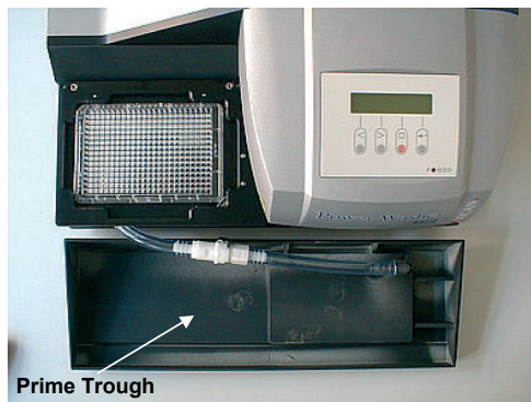
Figure 7-2 Removing the Prime Trough
