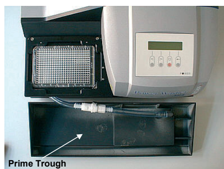
Figure 3-4 Removing the Prime Trough
