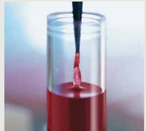
Tip occlusion alert by capacitive liquid level detection
